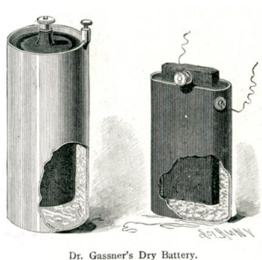
Figure 15 Pile sèche de Gassner, ~1890 ©JENSEN William B., p.3
